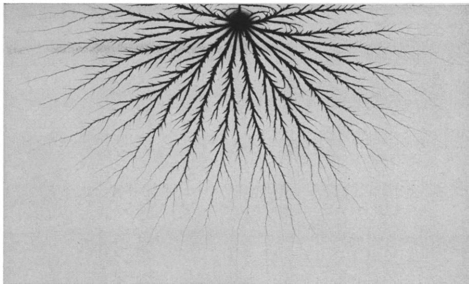
Fig. 8. Autograph of a streamer branching on a film in the plane of the point axis. The streamer came from a positive-potential pulse of about 40 kv, of rise time  $2 \times 10^{-8}$  second but of  $100\text{-}\mu\text{sec}$  duration, with gradual decline. [W. P. Winn and G. A. Dawson]
