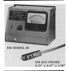
Seven full-scale ranges from  $2.5 \times 10^3$  to  $2.5 \times 10^6$  ergs/cm<sup>2</sup>-sec (0.25 to 250 MW/cm<sup>2</sup>).
