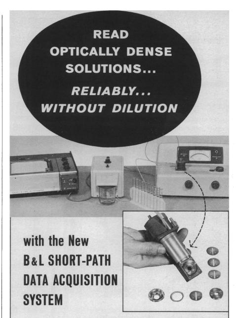
Samples that are too dark or too dense for conventional spectrophotometric readings can now be handled reliably, rapidly, and routinely. Gone is the necessity for time-consuming, error-prone dilutions. The newly developed short-path Flow-Thru Cuvette saves time and trouble. It has a short-path length capability between 0.1mm and 1.0mm . . . provided by an easily interchangeable stainless steel shim. Available shims provide path lengths of 0.1mm, 0.2mm, 0.5mm and 1.0mm.
