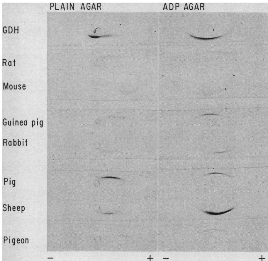
Fig. 1. Immunoelectrophoresis of GDH from different sources. The experiments were carried out in plain and ADP-containing agar with 0.05M veronal buffer, pH 8.2. All specimens were subjected to electrophoresis simultaneously (200 v, 135 min) on two large agar plates. Precipitin lines were stained for GDH activity.
