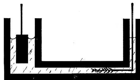
Fig. 1. Dendritic growth in a capillary tube.
