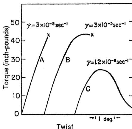
Fig. 4. Torque-twist curves for polycrystalline specimens of  $\text{Al}_2\text{O}_3$  at  $1200^\circ\text{F}$ , showing brittle fracture (*A*) and creep fracture (*B* and *C*).
