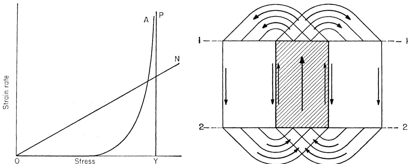
Figs. 1 and 2. Fig. 1 (left). Dependence of the shear stress upon the rate of shear strain in Newtonian viscosity (*ON*), in Andradean viscosity (hot creep of crystalline materials) (*OA*), and in ideal plasticity (*OYP*). Fig. 2 (right). Convection in a plastic space, due to the presence of a prism of higher temperature (shaded area).
