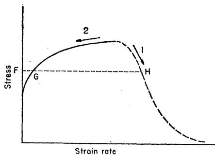
Fig. 5. Schematic curve for stress versus strain rate, illustrating the instability of hot creep. When the creep rate in the shear layer has risen to *FH*, it has fallen to *FG* elsewhere.
