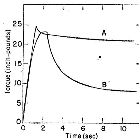
Fig. 6. Torsional creep relaxation in polycrystalline  $\text{Al}_2\text{O}_3$  with impurity content of (A) 0.2 percent and (B) 0.7 percent.
