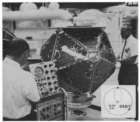
At TRW Space Technology Laboratories — in preflight testing under simulated space conditions—engineers use a Tektronix Oscilloscope to check performance characteristics of a nuclear detection satellite. Designed and built by STL for Air Force-ARPA, these icosahedronshaped satellites travel in pairs around the earth to detect nuclear explosions in space.
