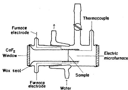
Fig. 2. Schematic diagram of cell for infrared study of chemisorbed molecules. [From Courtois and Teichner (10), with permission]
