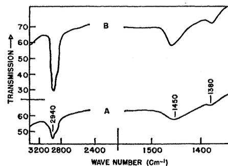
Fig. 3. A, Spectrum of acetylene chemisorbed on nickel; B, spectrum after treatment of chemisorbed acetylene with hydrogen at room temperature. [From Eischens and Pliskin (13), with permission]
