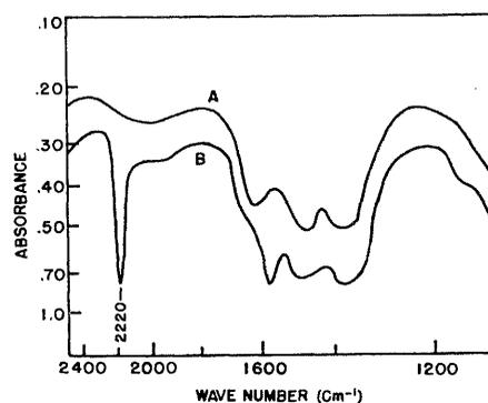
Fig. 6. A, Infrared spectrum of ZnO prior to reaction; B, spectrum 30 minutes after addition of  $0.01M$  formamide to the reaction mixture in the presence of air and light. [From A. Nergarian and M. C. Markham (21), with permission]
