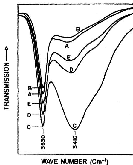
Fig. 1. Spectra of montmorillonite: A, dried at  $100^\circ\text{C}$  for 36 hours; B, dried at  $100^\circ\text{C}$  for 42 hours; C, after exposure to air saturated with water vapor; D, redried at  $110^\circ\text{C}$  for 6 hours; E, redried at  $100^\circ\text{C}$  for an additional 24 hours. [From Buswell, Krebs, and Rodebush (1), with permission]
