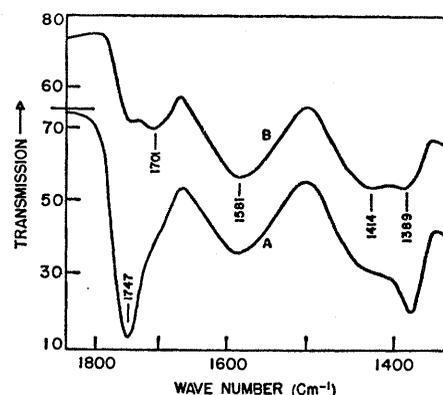
Fig. 7. Spectrum of acetic acid chemisorbed on  $\text{MgO-SiO}_2$ : A, at 70°C after drying of  $\text{MgO-SiO}_2$  at 400°C; B, after admission of water vapor at 70°C.
