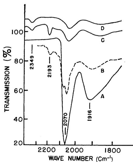
Fig. 5. Infrared spectroscopy study of the oxidation of CO: A, chemisorbed CO; B and C, intermediate stages after the addition of oxygen; D, spectrum after termination of the reaction. [From Eischens and Pliskin (17), with permission]
