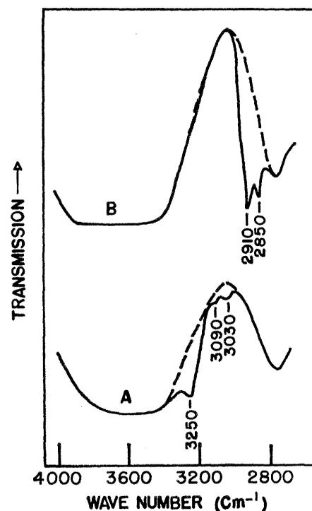
Fig. 4. A, Spectrum of acetylene chemisorbed on palladium; B, spectrum after treatment of chemisorbed acetylene with hydrogen at room temperature. [From Little, Sheppard, and Yates (14), with permission]
