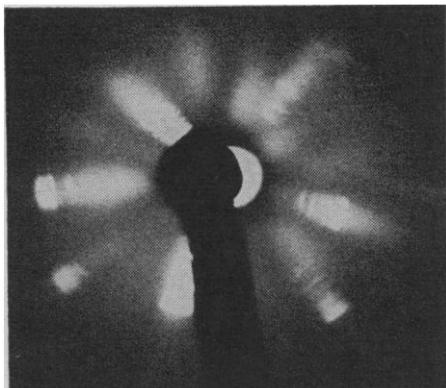
Fig. 3. Laue photograph of 1.5-cm thick potassium single crystal with appreciable orientation spread; 125 kv, 5 ma, 20 minutes, 10 cm between slit and film.
