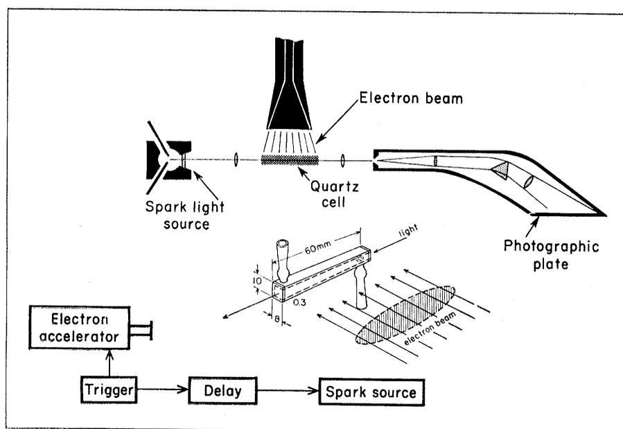
Fig. 3. Schematic diagram of apparatus used for kinetic absorption spectroscopy (16). Insert shows the construction of the absorption cell in greater detail.
