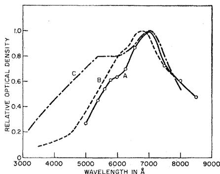
Fig. 6. Absorption spectra of hydrated and solvated electrons in (A) pure water irradiated by means of an electron pulse (14); (B) potassium chloride solution photolyzed by a light flash (23); (C) ethyl alcohol irradiated by means of an electron pulse (25).
