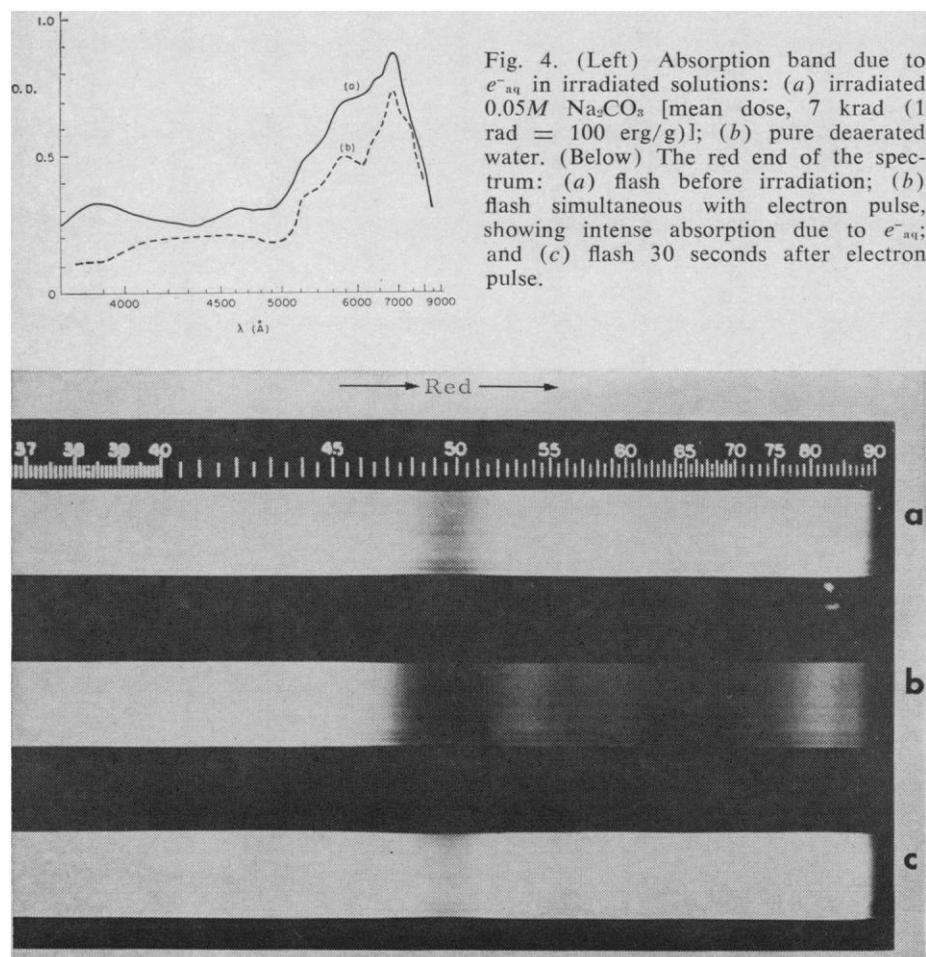
Fig. 4. (Left) Absorption band due to  $e^-_{aq}$  in irradiated solutions: (a) irradiated 0.05M  $Na_2CO_3$  [mean dose, 7 krad (1 rad = 100 erg/g)]; (b) pure deaerated water. (Below) The red end of the spectrum: (a) flash before irradiation; (b) flash simultaneous with electron pulse, showing intense absorption due to  $e^-_{aq}$ ; and (c) flash 30 seconds after electron pulse.
