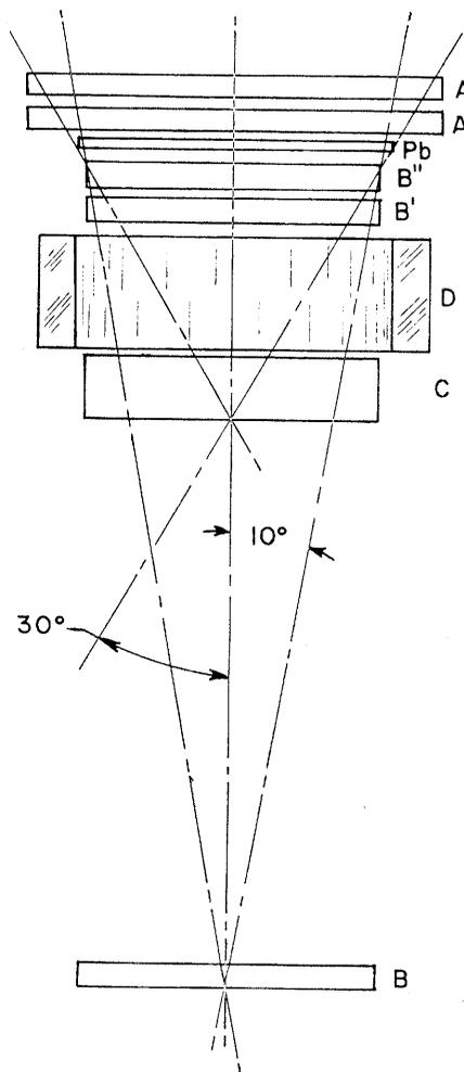
Fig. 5. Schematic diagram of the counter for measuring high-energy gamma rays. It was flown by the Rochester group in September 1963.
