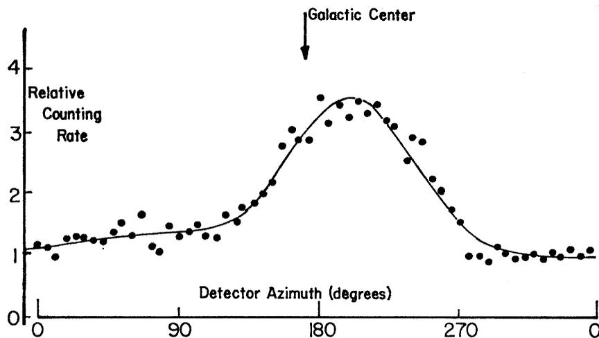
Fig. 2. X-rays detected by counters in a rocket, plotted against angle of spin about the axis of the rocket.
