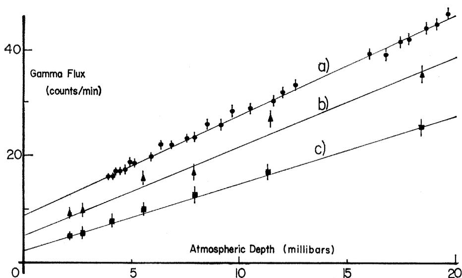
Fig. 6. Dependence of counting rates for high-energy gamma radiation, in a 30-degree cone, on thickness of air near the top of the atmosphere. Data for set *a* are from four early flights (27); data for set *b* are from the counter of Fig. 5 with the guard ring *D* not operating; data for set *c* were obtained by rejecting events that trigger *D*.
