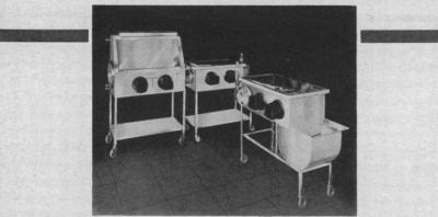
These units were designed for germ-free research procedures used in the world's most advanced laboratories. All metal parts are of life-long corrosion-resistant stainless steel.
