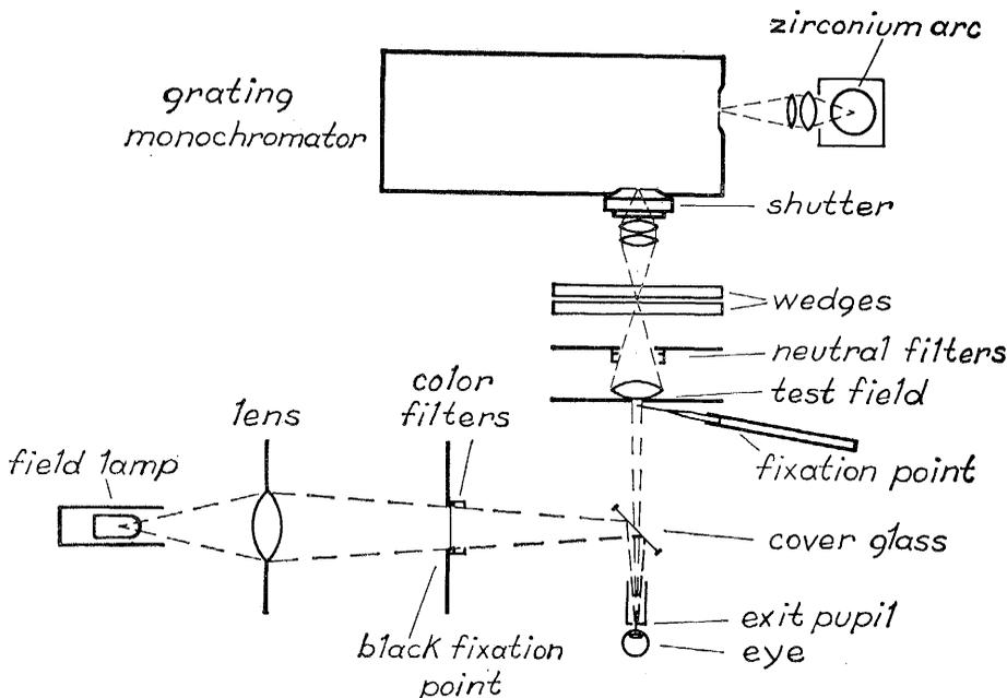
Fig. 1. Arrangement of the apparatus. It consists essentially of two light paths, one for presenting monochromatic test flashes of graded intensity, superimposed on steady colored backgrounds provided through the other light path. Both the test and background fields are seen in Maxwellian view.
