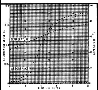
Portion of DNA-RNA thermal denaturation record, made with Gilford 2000 Spectrophotometer and Linear Thermosensor, illustrates linear recording of absorbance and temperature on same chart. Another use for the 2000—one versatile system adaptable to column chromatography, enzyme kinetics, sucrose density gradients, amino acid analyses . . . or your area of research.
