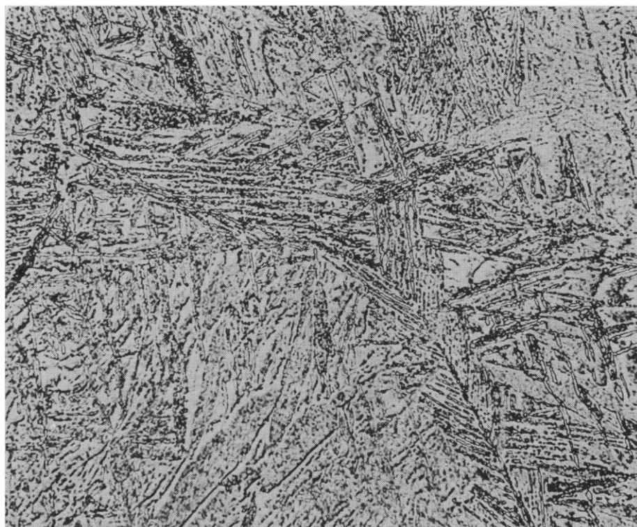
Fig. 1. Ordered lamellae of the hexagonal, high-density form of Mg_2Si , formed from a dendrite of normal material in a field of excess silicon. Reaction conditions were 900°C, 30 kb for 5 minutes. The specimen was deliberately held below its melting point during this experiment.
