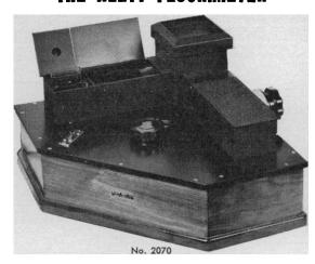
Designed for the rapid and accurate determination of thiamin, riboflavin, and other substances which fluoresce in solution. The sensitivity and stability are such that it has been found particularly useful in determining very small amounts of these substances.
