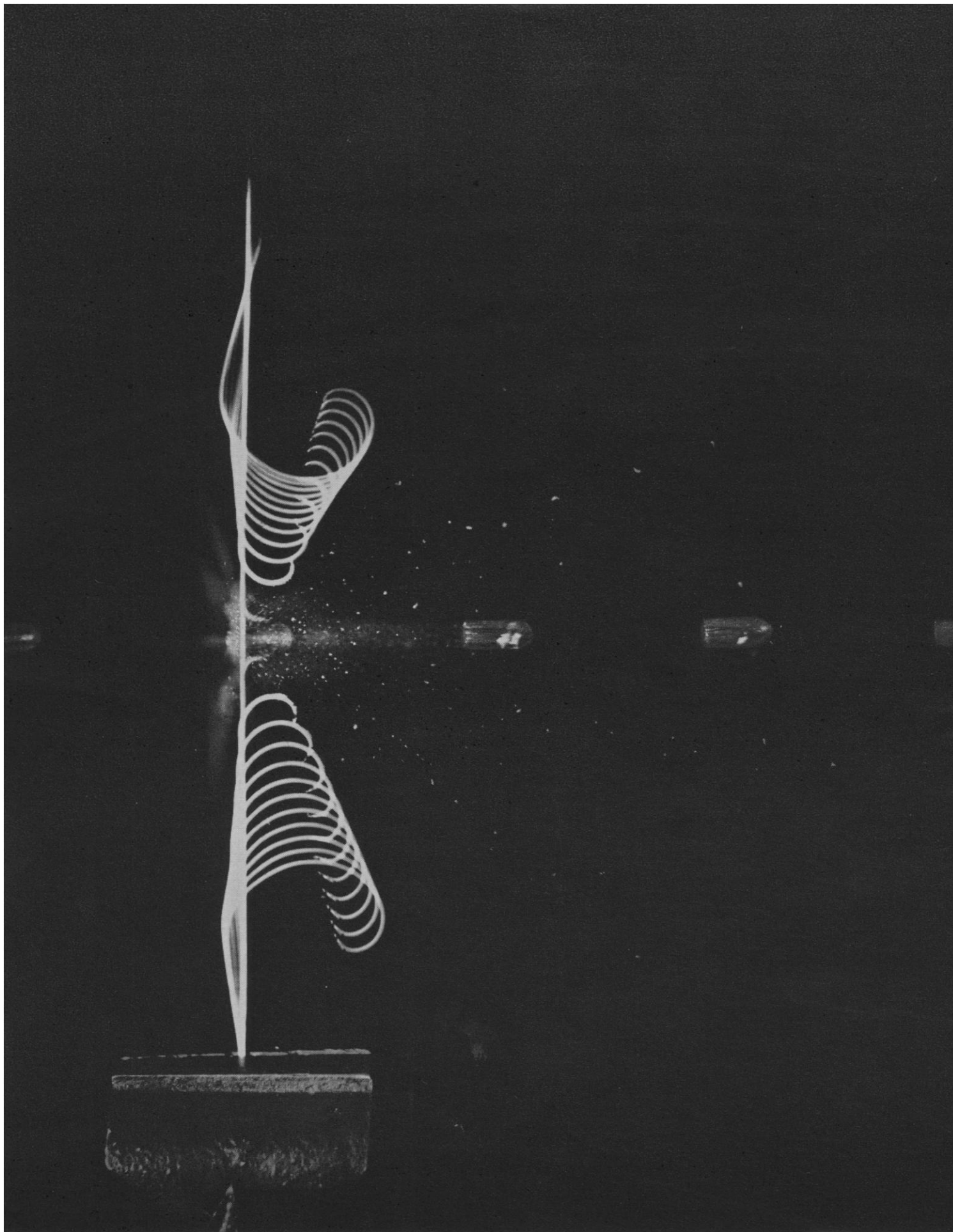
Dr. Harold Edgerton had a fully developed positive and a negative just 20 seconds after he took this multiple exposure of a .22 caliber bullet cutting a single copper wire. He used his new EG&G Multiple Microflash® unit with a Speed Graphic loaded with Polaroid P/N 4x5 film.
