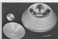
BR-4 Two-Liter General-Purpose Rotor (with stainless steel cups & screw covers)
