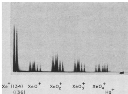
Fig. 1. Mass spectrum of xenon tetroxide.
