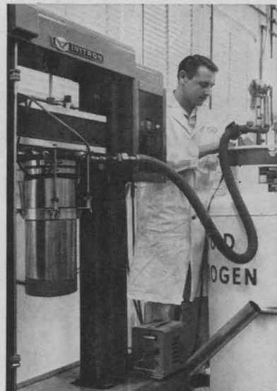
Special cryostat and system installed on an Instron Test Instrument for a test at -423°F.
