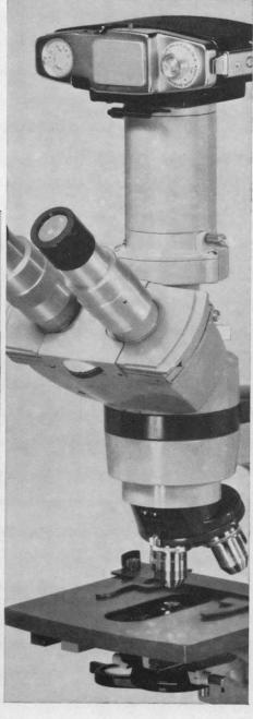
Your choice of new Polaroid®† film pack back or 35 mm with two magnifications — 2.8X and 5X. Both camera backs used interchangeably with the same lens/shutter assembly. New Microstar also accommodates the famous AO 682 Camera.
