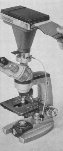
Camera work is easier, too. Visual and photomicrographic systems are parfocal...you just focus the specimen through the eyepieces and snap the shutter. Field coverage and film magnification remain constant regardless of changes in interpupillary settings. No compensations to make.
