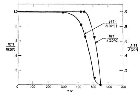
Fig. 1. Effect of annealing for 1 hour at a temperature  $T$  on the average length,  $l$ , and density,  $N$ , of etched tracks in muscovite from Renfrew County, Canada. In the graph,  $l$  and  $N$  are normalized to the average length and density measured with no heat treatment.
