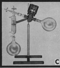
To evaporate aqueous solutions, high-boiling-point solvents, strong acids, alkalis and radioactive materials without contaminating back-drip.
