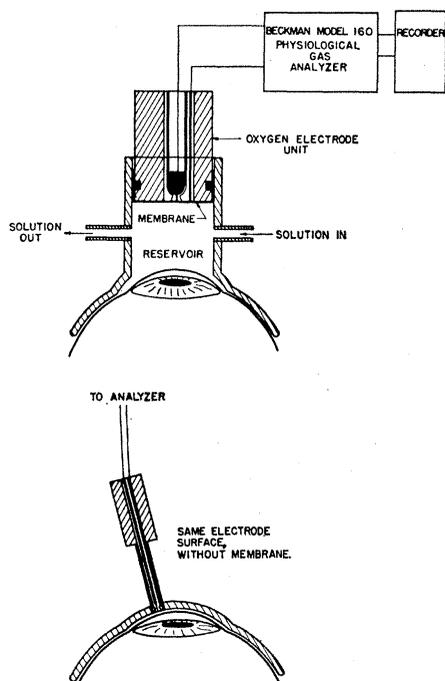
Fig. 1. Schematic diagram of the electrode and lens assemblies used to obtain data for calculating the rate of oxygen consumption by the cornea in vivo. (Top) The reservoir volume may be changed as desired by moving the electrode assembly. (Bottom) The volume of the reservoir is at its minimum—that is, the clearance is normal for a scleral contact lens; the electrode is used without a membrane in this bottom assembly.
