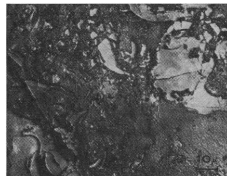
Fig. 1. Micrograph of high pressure zirconium oxide ( \times 2000 ). White grains are tetragonal phase in monoclinic matrix.
