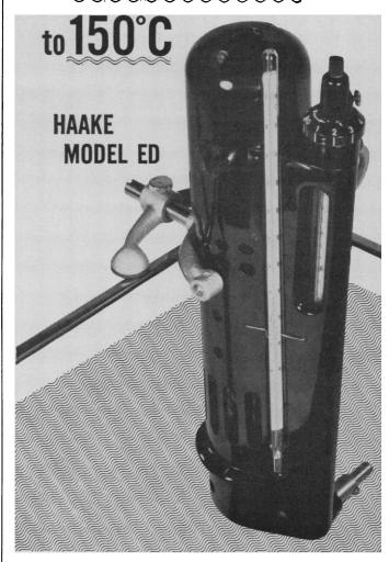
The Haake constant temperature circulator Model ED may be used either to maintain accurate temperature control of any open bath (stirring) or for control by pumping through externally mounted appliances (circulating) such as spectrophotometers, refractometers, polarimeters, titration vessels, etc.
