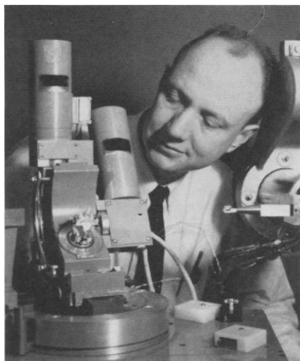
X-rays, from the device at the right in this picture, strike against a crystal sample held in the goniometer, left. A geiger counter measures intensity of refracted X-rays.
