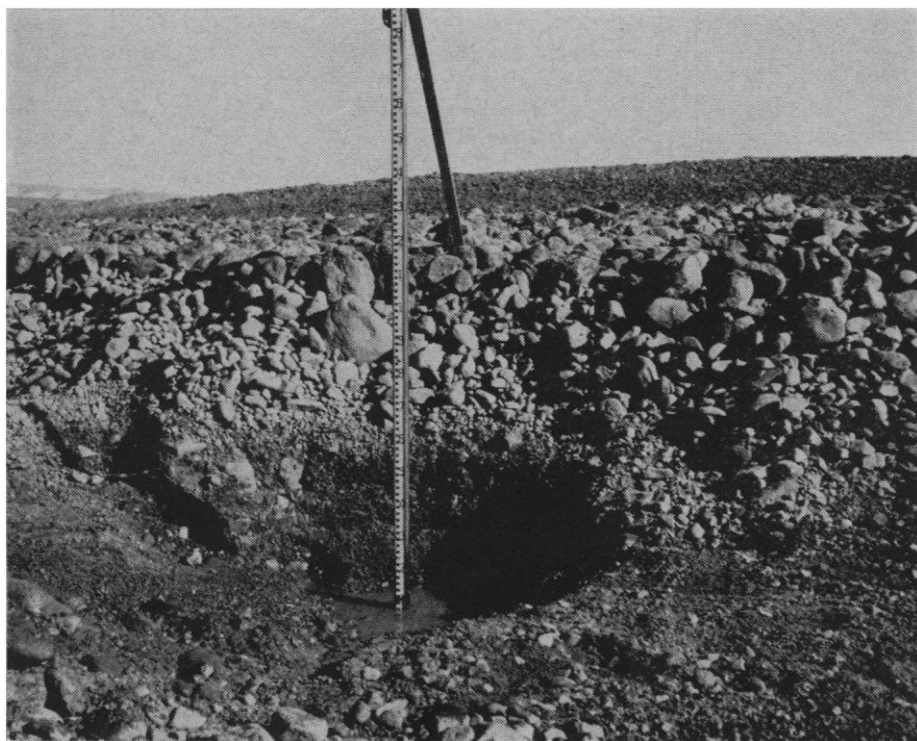
Fig. 2. Profile of vertical sorting in flat terrain in which a "boulder field" is forming (Thule area). The scale rests at 25 cm below the level of perennially frozen ground.
