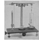
**5** Specific-gravity chain balance— Model S100—Ideally suited for S.G. determinations of liquids and solids to within 0.0001. Also operates as a sensitive chain analytical balance. From \$168.
