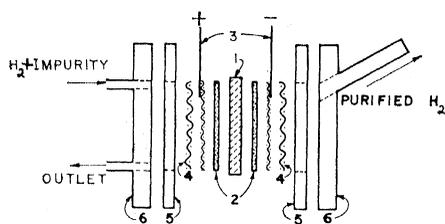
Fig. 1. Exploded section of model hydrogen purification cell: 1, saturated filter paper or membrane; 2, electrodes; 3, potential delivery screens; 4, spacers; 5, gaskets; 6, plastic casing.
