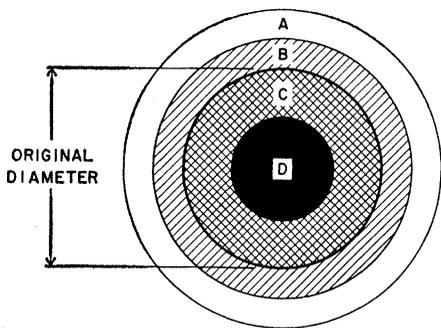
Fig. 2. Schematic cross-sectional cut of a silver coil based on the different strata observed and the conditions indicated by analytical results: *A*, Calcium carbonate redeposited from limestone by the reaction of atmospheric  $\text{CO}_2$  and water. *B*, Calcium carbonate with AgCl and elements that have diffused out of the original silver. *C*, Silver chloride, metallic silver, and elements that are replacing the original silver. *D*, Remaining original silver.
