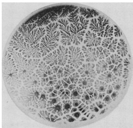
Fig. 2. The coalescence of many separate cavities into one circular cavity. The residual oil appears in the form of filaments throughout the cavity area.
