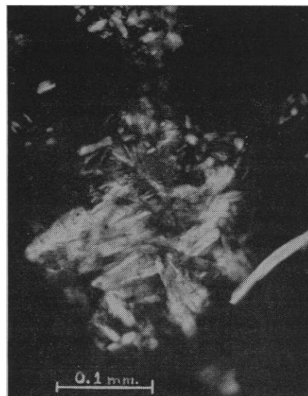
Fig. 1. Aggregates of crystals of the metastable hexagonal modification of RbAlSi_3O_8 . Polarized light, Nicol prisms crossed.
