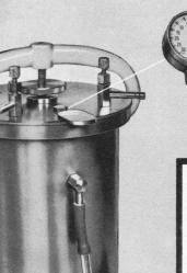
The corrosion-resistant, stainless steel construction of the new Torbal B.T.L. anaerobic, jar avoids the dangers inherent in glass jars. It is a simple but effective apparatus for producing anaerobic conditions, using a patented room temperature catalyst, which completely eliminates the need for electrical or auxiliary heating. Growth of anaerobes is safer, easier and quicker. For complete data write for Bulletin Torbal AJ. The Torsion Balance Company
