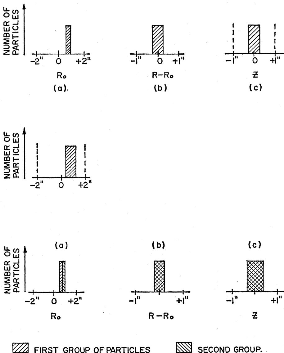
Fig. 3 (top). *a*, Distribution of particles in closed-orbit radius ( $R_0$ ); *b*, radial betatron oscillation amplitude ( $R-R_0$ ); *c*, vertical betatron oscillation amplitude ( $Z$ ). In each graph, 0 is at the center of the vacuum chamber. Fig. 4 (middle). Actual radial positions in the storage-ring vacuum chamber for the particles of Fig. 3. Fig. 5 (bottom). Stacking of two groups of particles brought to full energy in two different cycles of the accelerator.
