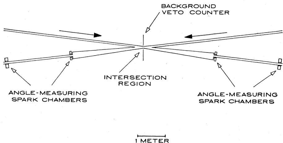
Fig. 7. Experimental arrangement for a 62-Gev proton-proton colliding-beam scattering experiment.
