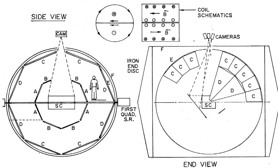
Fig. 9. Apparatus for a 62-GeV experiment on reactions leading to the production of new particles or resonances. SC, Main spark chamber; A, Sagitta spark chambers,  $\theta < 45^\circ$ ; B, Sagitta spark chambers,  $\theta > 45^\circ$ ; C, end-point spark chambers,  $\theta > 45^\circ$ ; D, end-point spark chambers,  $\theta < 45^\circ$ ; E, sphere of time-of-flight counters; F, analyzing magnet coils.
