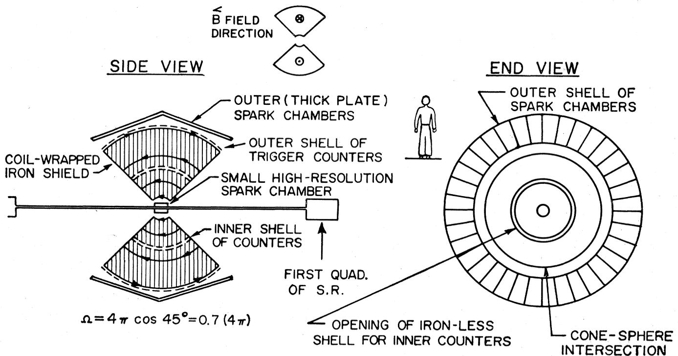
Fig. 10. Arrangement for a 62-GeV experiment on a short-lived intermediate particle decaying into a  $\mu$ -meson and a neutrino.
