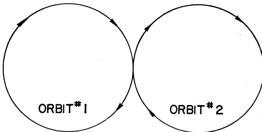
Fig. 1. Basic colliding-beam arrangement.
