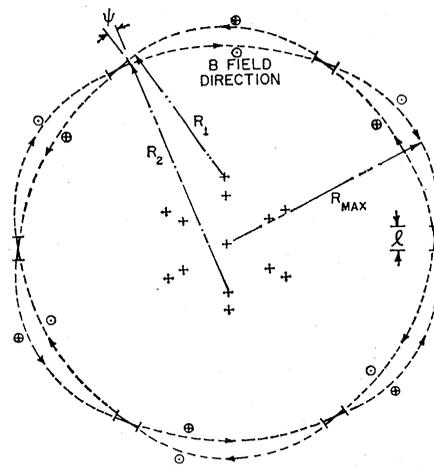
Fig. 6. Orbits of protons in a concentric storage ring. This design provides six interaction regions, at all of which experiments could be simultaneously carried on.
