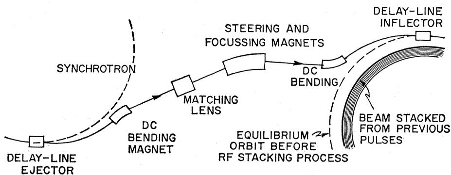
Fig. 2. Transfer from synchrotron to storage ring.
