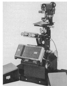
Features include: Phase and Anoptral Contrast Microscopy Fluorescence Microscopy Cinephotomicrography and Time Lapse System Photomicrography with Polaroid and 35 mm cameras Choice of five light sources
