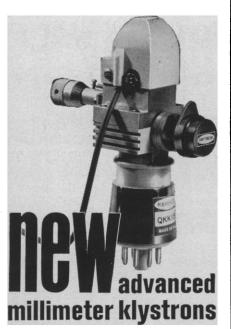
Now available...improved and rugged...50 Gc to 101 Gc klystrons featuring uniform output power and exceptional frequency stability throughout 500-hour warranty life. Thermal stability is  $-4MC/^{\circ}C$ . max. to 83 Gc ( $-6MC/^{\circ}C$ .max. above 83 Gc). Compatible voltages including 6.3V heaters simplify power supply requirements. Actual power outputs are well above rated minimum.
