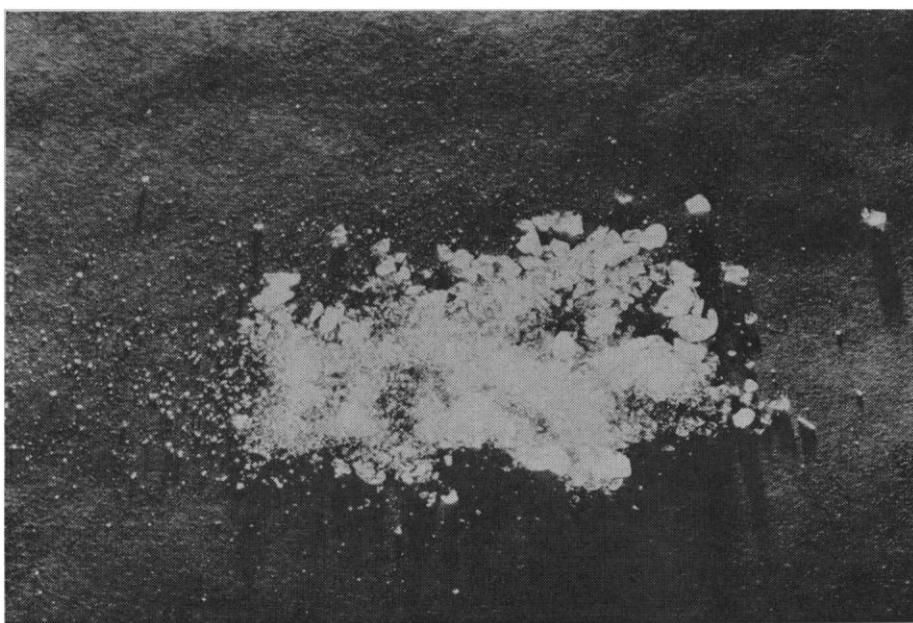
Fig. 2. Fragments of broken Prince Rupert drop.
