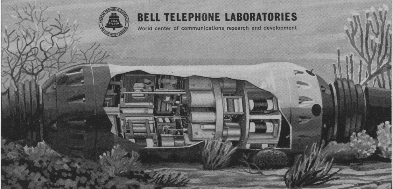
View of deep-sea amplifier with casing cut away. The casing is of noncorrosive beryllium copper, tested to withstand pressures up to 11,000 psi.
