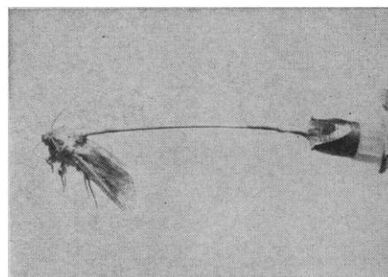
Fig. 1. Moth preparation for the study of activation of wing beat by low-intensity x-rays. The attachment of the subject to the crystal transducer can be seen.
