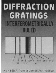
Ag 4358 A from a Jarrell-Ash replica of MIT master (14th order), 11-Meter Spectrograph. Res. better than 750,000.
