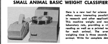
Here is a new tool for science that offers many interesting possibilities in research and other applications. This machine weighs and records laboratory rats, providing a visual reading as well as a printed record each animal. The average weighing time is three seconds per animal. Write for complete details.
