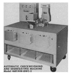
Laboratory animals, such as rats, are weighed, classified and segregated into three separate cages of predetermined weight groups with this new time-saving machine—the Exact Weight Small Animal Automatic Checkweigher.
