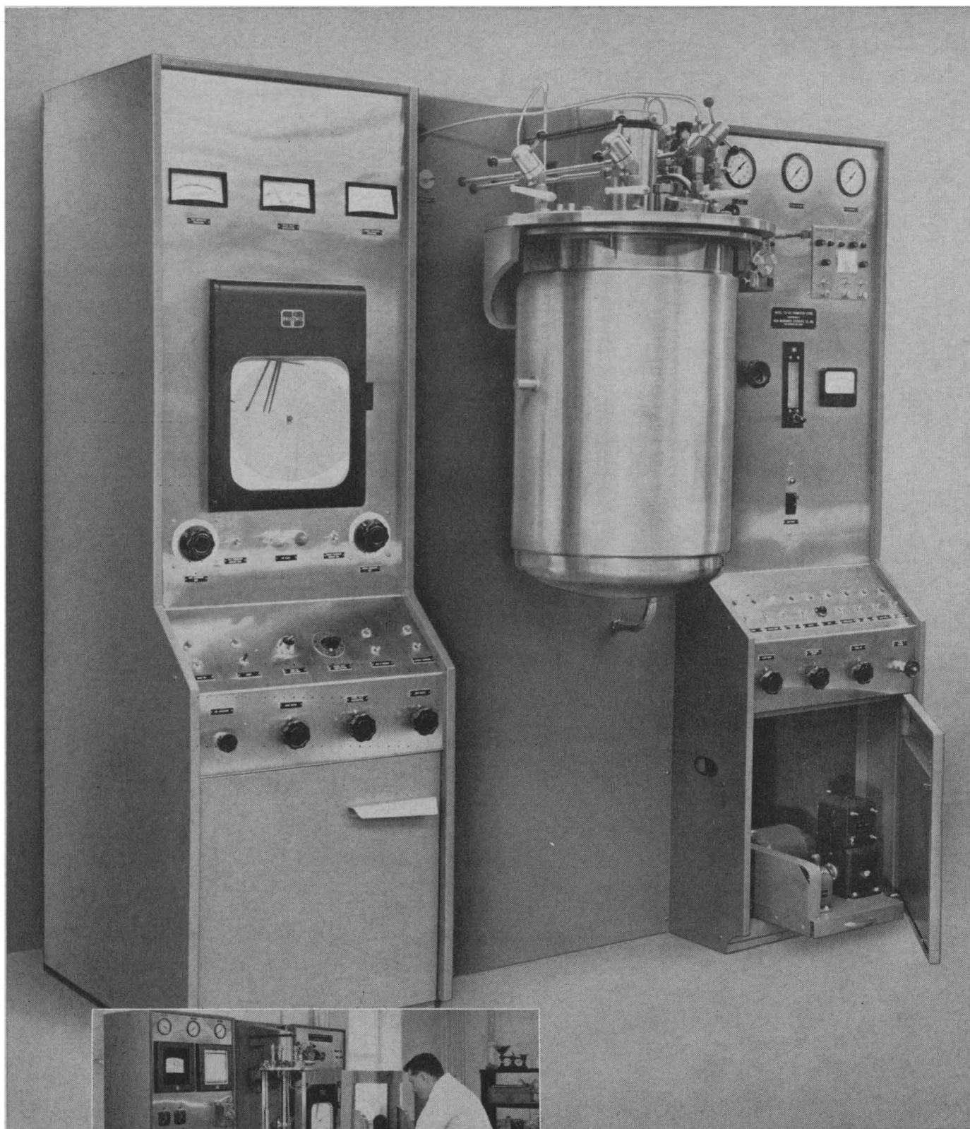
130 Liter Continuous Culture Apparatus: Model CF-130 has 2 Variable Speed Tubing Pumps (behind front doors) which are set for desired rate of feed and automatic harvesting, while constant working volume is maintained. Portable stand (not shown) brings operator to convenient working height.
