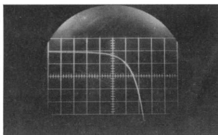
Fig. 1. Decay curve at secondary coil with sample of metallic InSb as a core at a temperature of 4.2°K. Decay is indicative of a sample of very high conductivity, comparable to that of pure tin or indium above their transition temperatures. The vertical scale shows voltage, the horizontal shows time.
