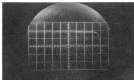
Fig. 2. Decay curve at secondary coil with same sample at 1.3°K after complete transition to the superconducting state.
