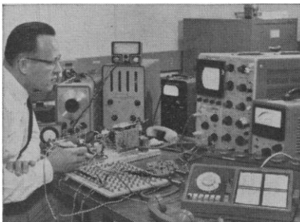
Indianapolis Laboratory, Ind. We were perfecting improved automatic dialer telephones. One model will permit the customer himself to record 50 frequently called names and numbers and then dial by simply selecting a name and pressing a button.
