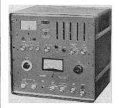
LYRA SYSTEM is a versatile single channel spectrometry system which offers both scaler and ratemeter read-out. It consists of Model SM-10 Single Channel Spectrometer and Model DS-5B Decade Scaler with high voltage supply.
