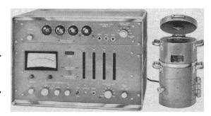
ARCTURUS SYSTEM is a completely automatic scanning spectrometry system and provides a permanent record of the spectrum. It is composed of Model SM-10 Single Channel Spectrometer, Model RHV-1B High Voltage Supply, Model SS-30 Mechanical Spectrum Scanner, and a Strip Chart Recorder.
