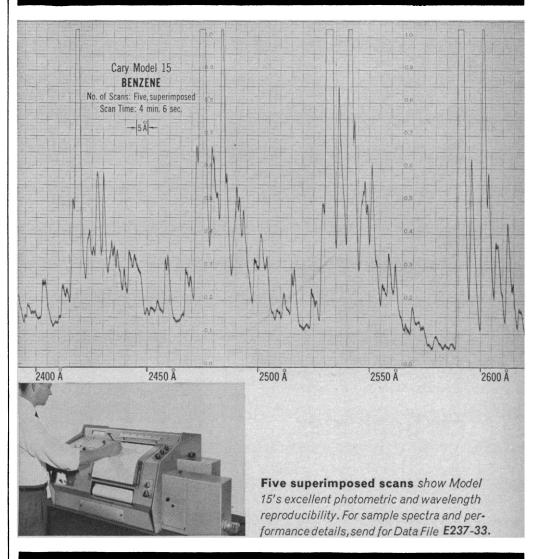
Traditional Cary performance is built in. Advanced design provides precision and reliability over 1750-8000  $\mathring{A}$  range: At 1850  $\mathring{A}$ , near zero absorbance, photometric accuracy is 0.002 with 0.3  $\mathring{A}$  resolution...even at 2.0 absorbance, photometric accuracy is 0.008 with 3  $\mathring{A}$  resolution.
