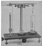
3. Specific-gravity chain balance— Model \$100—Ideally suited for S.G. determinations of liquids and solids to within 0.0001. Also operates as a sensitive chain analytical balance. From \$168.
