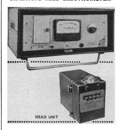
The newest Vibrating Reed Electrometer Type N616B measures direct currents down to -10<sup>15</sup> amps full scale using internal resistance! Very low noise and drift—±100 Microvolts over 24 hours. Applied D.C. is converted to A.C. by a vibrating reed capacitor and amplified by a stable A.C. amplifier. Output meter calibrated in voltage plus recorder output facility. Proven performance at low cost!
