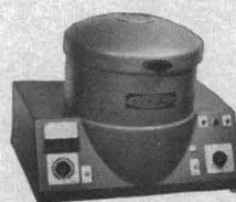
SS-3 Automatic Superspeed Centrifuge* — 17,000 rpm — 34,800 x G with push-button simplicity and armor-plate safety
