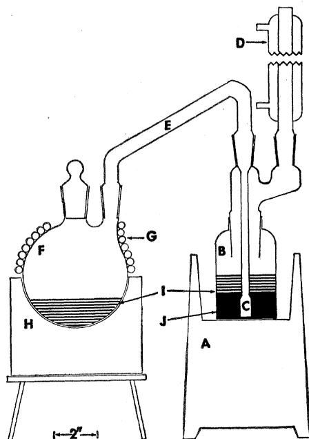
Fig. 1. Cross section of the new extractor: *A*, ultrasonic bath or suitable support; *B*, polyethylene or glass extraction flask; *C*, sintered-glass filter; *D*, condenser; *E*, glass connecting tube; *F*, solvent flask; *G*, cooling coils; *H*, heating mantle; *I*, solvent; *J*, material being extracted.
