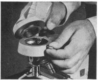
Interchangeable, Rotatable Bodies Your choice of interchangeable, rotatable, monocular of thinocular or trinocular bodies. Simply loosen thumb screw to rotate (full 360°) or interchange. Special inclined monocular body with vertical photographic tube also available.
